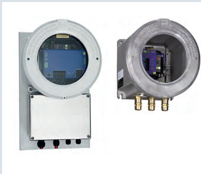
R. STAHL's UPS solutions with capacitors for energy storage are available as ATEX/IECEx models with combined Ex de ignition protection (left), and in various regional versions, for instance in Ex d enclosures with an NEC® certificate (right image)
