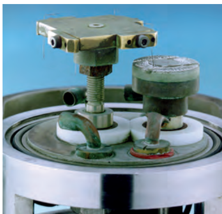
FIGURE 2 Contact array of the spark test apparatus according to IEC 60079-11
