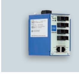
The 9721 switch is used for linking electrical Ethernet networks with optical 100 Mbit/s Ethernet networks. The 4 FO ports are designed for operation in the hazardous areas with the "op is" type of protection. This way, conventional fibre optic cables can also be used in hazardous areas and may be connected and disconnected during operation (hot-swap).
