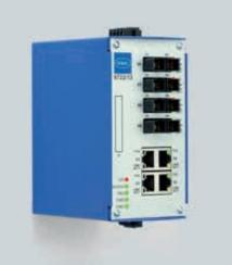
The series 9722 managed 100 Mbit/s switches are specifically designed for use in PROFINET networks. They feature ring functionality based on the Media Redundancy Protocol. The 4 FO ports are designed with the "op is" type of protection, making maintenance of the devices in Zones 0, 1 and 2 easy (hot swap, hot plug).
