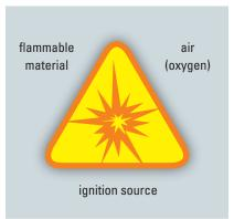
Fig. 1: For an explosion to take place, these three factors need to be present at the same time
