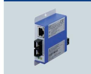
The 9721 series media converter converts electrical signals into optically inherently safe "op is" signals, allowing installation and maintenance work to be conducted on fibre optics in Zones 0, 1 and 2 without the need for downtime (hot swap/ hot work). It is particularly suitable for the IS1+ Ethernet Remote I/O System.
