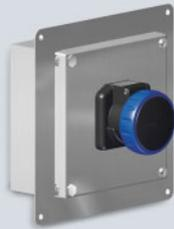
Size 1 socket outlet assemblies (176.5 x 176.5 mm) for use in clean rooms with a socket flange for voltages of up to 277 V/16 A. The built-in sockets meet very stringent requirements in terms of surface texture and electrostatic charge, which means that the accumulation of particles (dust) is kept to a minimum.
