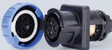
3-pole 16 A compact flange socket for voltages of up to 277 V; for installation directly into enclosures for Zones 1/2 and 21/22. Integrated rotary switch mechanism with full AC-3 switching capacity in accordance with IEC/EN60947-3.
