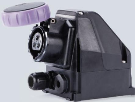
The 2-pole and 3-pole socket for extra-low voltages of up to 50 V/16 A; suitable for use in Zones 1/2 and 21/22. The enclosures are made in 2-component technology, and an excellent degree of protection, IP66, is guaranteed, whatever the working environment. High-quality plastics for an extreme operating temperature range of between –60 °C and +55 °C.
