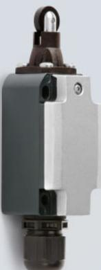
Metal position switch; switch dimensions meet the requirements of DIN EN 50041. The field of application and requirements are the same as for the 8060/2 series standard-compliant position switch.
