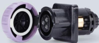
The 2-pole and 3-pole 16 A flange socket for extra-low voltages of up to 50 V/16 A; suitable for use in Zones 1/2 and 21/22. High-quality, self-cleaning contact materials ensure optimal contact. Non-wearing, self-cleaning lamellar contact technology ensures that contact resistances are low.
