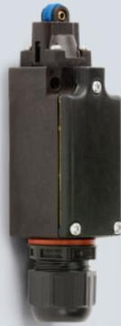
Plastic Position switch; switch dimensions meet the requirements of DIN EN 50047. It is designed to detect the position of moving components. Certified versions fulfil the requirements for safety switches as set out in EN 13849-1 and have positive-opening contacts in accordance with EN 60947-5-1.
