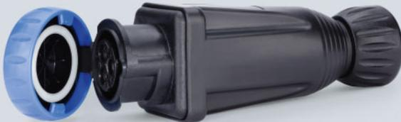
3-pole 16 A compact coupling for voltages of up to 277 V; allows direct installation of flexible cables. The reliable internal strain relief and impressively effective sealing system make this coupling well suited to mobile use.
