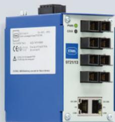
These switches transform electrical (TX) into optically inherently safe (op is) Ethernet networks. They allow installation and maintenance work to be conducted on fibre optics in Zones 0, 1 and 2 without the need for downtime (hot swap/hot work). They are suitable for systems such as IS1+ Ethernet Remote I/O, HMI and camera systems.
