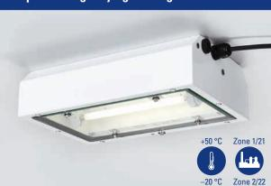
The 6118 series single-lamp compact emergency luminaire is made from powder-coated sheet steel or V4A stainless steel and is ideal for spay booths, paint shops and clean rooms. If used in conjunction with symbols or other markings, they can be used as illuminated signs or escape route luminaires. The integrated battery will power the luminaire for 1.5 or 3 hours. The luminaire automatically conducts a weekly functional test.
