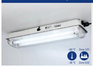
This light fitting is suitable for both standard lighting applications and emergency lighting applications in virtually any facility. With very little effort, using the accessories it can be fitted to the wall, ceiling or a pole or, alternatively, it can be suspended. The practical central lock has a safety switch that disconnects the power supply at all poles when the plastic enclosure is opened.
