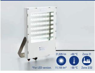
The 6525 series LED floodlight is ideal for lighting up large areas from elevated positions. Its wide-beam light distribution make it an excellent choice as a spotlight for lighting industrial buildings or as a high-bay light fitting; it can also be installed in relatively inaccessible places. The floodlight is generally designed with an enclosure and a bracket made from single-coated sheet steel.
