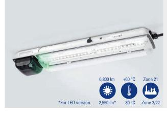
EXLUX 6409 series luminaires are perfect for emergency lighting applications (Zones 2 and 21). These luminaires provide lighting in accordance to the relevant standards for 90 or 180 minutes in the event of a power failure. With very little effort, these can be fitted to the wall, ceiling or a pole or, alternatively, be suspended. The LED technology boasts high luminous efficacy and longer service life.
