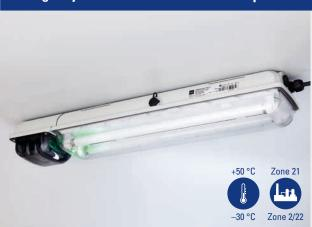
The EXLUX 6409 series is designed to provide emergency lighting. It is lightweight and requires little maintenance. An external battery will power the emergency lighting for 1.5 or 3 hours. If one lamp is faulty, the luminaire switches immediately to the working lamp. When the luminaire or battery case is opened, the battery circuit is disconnected. The robust plastic enclosure is easy to open thanks to the practical central lock.
