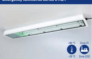
This sheet steel emergency luminaire has a variety of installation options. The integrated battery ensures that the emergency lighting lasts for up to 180 minutes. When the emergency lighting is in operation, if one fluorescent lamp is faulty, the luminaire automatically switches to the working lamp.
