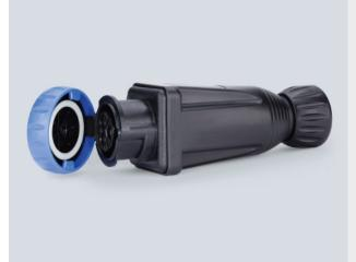
3-pole 16 A compact coupling for voltages of up to 277 V; allows direct installation of flexible cables. The reliable internal strain relief and impressively effective sealing system make this coupling well suited to mobile use.
