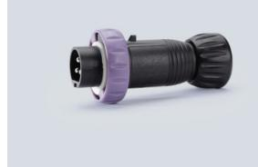
The 2- and 3-pole 16 A connector for extra-low voltages of up to 50 V/16 A. High-quality contact materials ensure optimal electric contact. Very little force required to plug and unplug thanks to the floating pins/connectors.
