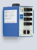
These switches transform electrical (TX) into optically inherently safe (op is) Ethernet networks. They allow installation and maintenance work to be conducted on fibre optics in Zones 0, 1 and 2 without the need for downtime (hot swap/hot work). They are suitable for systems such as IS1+ Ethernet Remote I/O, HMI and camera systems.
